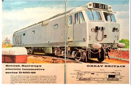
Line electrification north of Crewe, British Rail was unsure whether its existing 2 580 bhp Brush Class 47 diesel electrics would be reliable enough to work expresses to Glasgow and so fifty 2 700 horsepower English Electric Class 50 locomotives - numbered from 400 to 449 - were ordered and built in 1967 and 1968.
